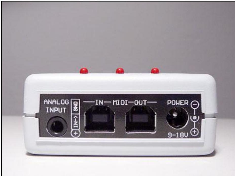
In the left side of the panel where is written “Analog Input”, usually you can connect some kind of analogue source. For example: a breath controller, foot pedal, potentiometer and etc. Polarity of connecting of the input connector is showed in the picture.
