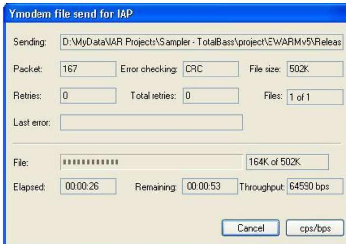
If the loading of the Bootloader is successful, on the computer screen in the window of Hyper Terminal should display a message similar to the following:
