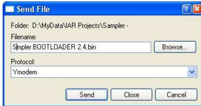
After selecting the file type and the protocol, you should press [Send] which starts loading of the **Bootloader**. On the computer screen should shows up another window that shows the status and progress of the loading. On the screen of the sampler will shows a message "**Loading ...**" and progress indicator that also shows the progress of the update. During loading the uppermost lamp L1 of the front panel of the sampler flashes.
