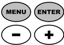
Then you should start the sampler in a special way to start the subroutine Firmware Loader, which helps to upgrade Bootloader. For this purpose, during power-up you have to press and hold simultaneously the buttons MENU and ENTER on the front panel of the sampler.
