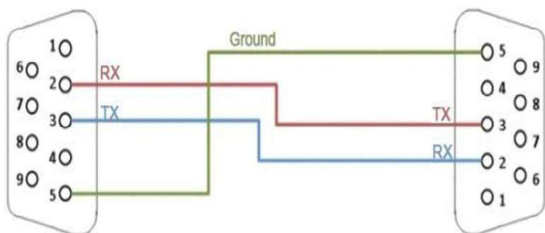
Picture and circuit diagram of the serial cable required for connection between a computer and a sampler.
